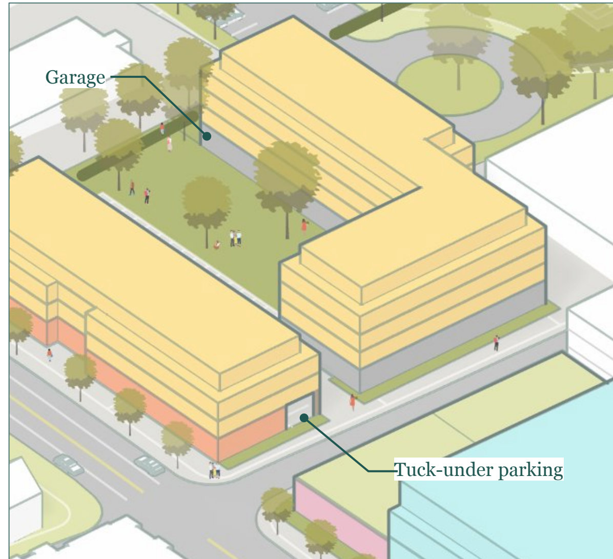
Tuck-under and enclosed parking accessed from Los Angeles St
