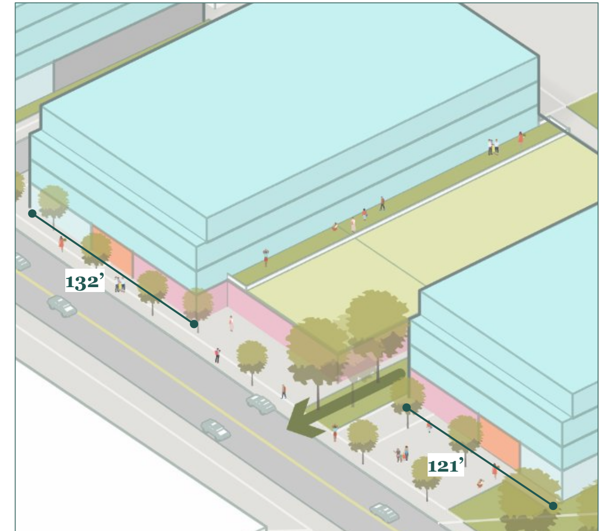
Offset in Commercial Building Facade
